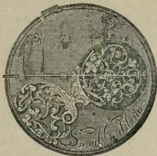
Fig. 5.—Hog's Bristle as a Balance Controller.
