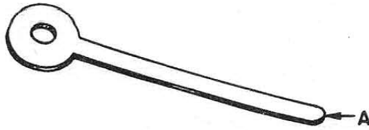
Seconds Wheel Tension Spring Assembly No. 7
