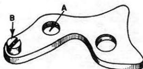
Hour Yoke Connecting Lever Assembly No. 10
