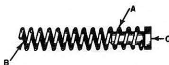
Push Piece for Setting Back to Zero Coil Spring and Plunger Assembly No. 2
